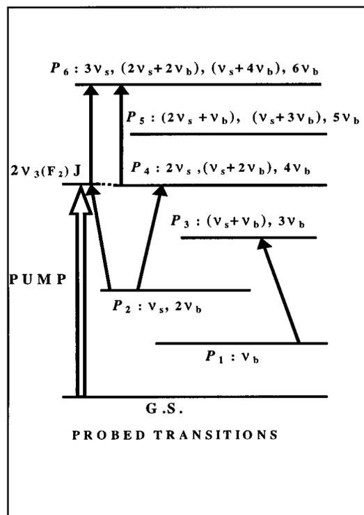
**Figure 2.** Simplified diagram of the CH<sub>4</sub> vibrational energy levels. These levels are gathered in polyads of interacting states. Each polyad  $P_N$  gathers all the states such as  $N = n_b + 2n_s$  where  $n_s$  and  $n_b$  are the numbers of stretching and bending excitation quanta. For instance, the pentad  $P_2: (\nu_s, 2\nu_b)$  gathers the  $\nu_1$  and  $\nu_3$  levels ( $n_s = 1$ ) and the  $2\nu_2$ ,  $2\nu_4$ , and  $\nu_2 + \nu_4$  levels ( $n_b = 2$ ).
