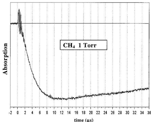
**Figure 3.** DR signal obtained by probing a diad  $\rightarrow$  octad transition at  $2949.11\text{ cm}^{-1}$  in methane at 1 Torr pressure. It shows a time decay in transmission of the probe beam due to an increase of population in the lower level of the probed transition, followed by a slow time rise back to equilibrium due to the V–T,R deexcitation of this level. This DR signal corresponds mainly to the time evolution of the populations in the states of the diad.
