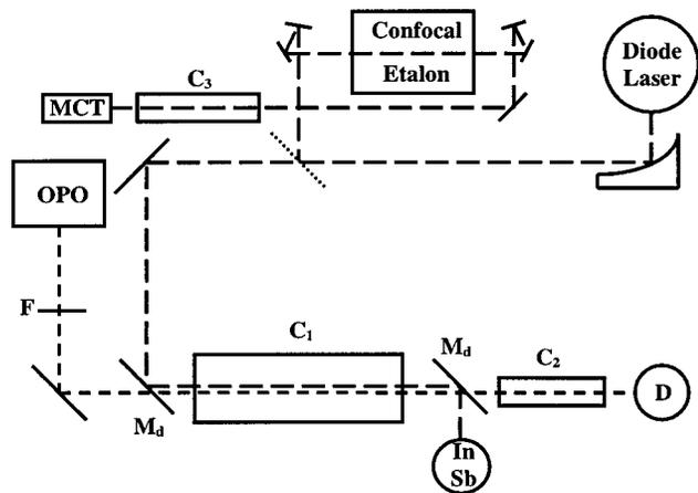
**Figure 1.** Schematic diagram of the experimental setup used for double resonance measurements in methane excited to  $2\nu_3(F_2)$  rovibrational levels by an optical parametric oscillator (OPO).  $C_1$  is the double resonance cell,  $C_2$  and  $C_3$  are absorption cells filled with CH<sub>4</sub> and C<sub>2</sub>H<sub>4</sub>, respectively,  $M_d$  are dichroic mirrors,  $F$  is a filter, and  $D$  is a pyroelectric detector.
